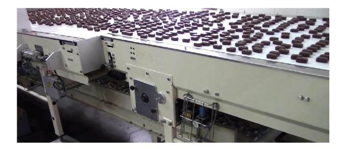
Conveyors take sweets from the production line, automatically distribute the flows of sweets depending on the load of the FlowPack machines. Pivoting belt conveyors provide uniform change of direction of the product row at an angle of 10  $^{\circ}$  –180  $^{\circ}$ .
